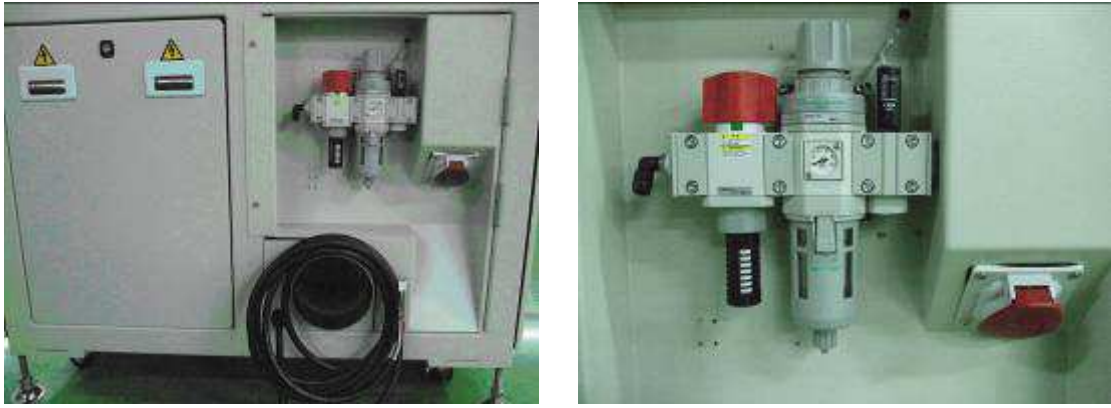
Figure 2.2 Compressed air connection and adjustment
